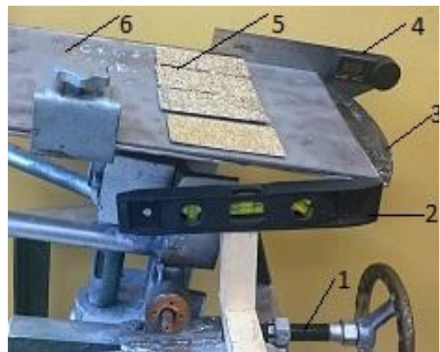
Fig. 3. Installation to determine the dynamic coefficients
